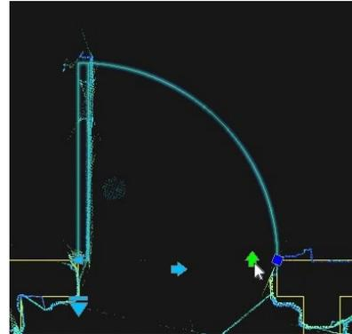
➤ To place the window to the existing opening, select Window (first, you must choose a line to align the window).
