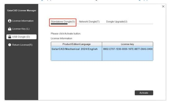
3. Click Activate button to finish the standalone dongle activation. Then restart your GstarCAD Mechanical 2024.
