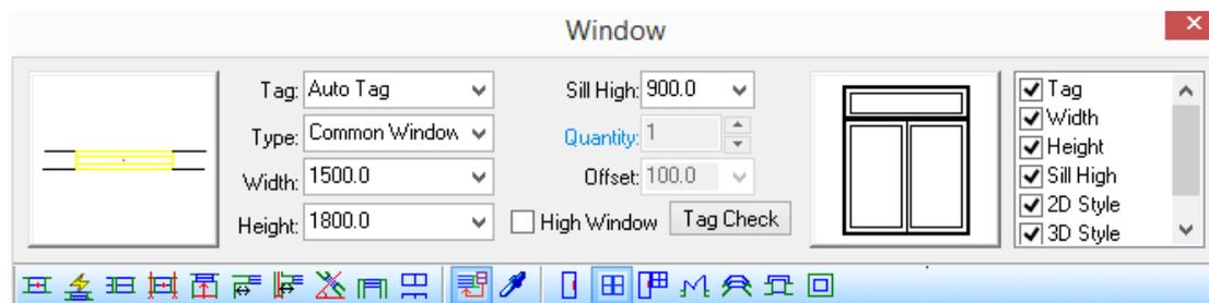
If user does not want to change some parameter during the replacing, please uncheck the related checkbox, after which, the parameter would remain unchanged and keep the same with that of the original drawing after the replacing. For example, if user does not want the width of the existing door to be changed when converting the door into a window, the "Width" check box should be unchecked.
