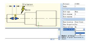
Save and exit the Block Editor, choose the Dynamic Block, you will find that one grip has disappeared. In fact, after changing the number of grips from "2" to "1", the first thing that disappeared was the basic grip of parameters, namely the first point when adding parameters.
