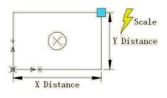
**3. Test the Dynamic Block:** After exiting the Block Editor, drag the grip of the top right corner of the rectangle, you can see the whole dynamic block is scaling as the grip is moving. It is easy to find that both the circle and the rectangle scale by the base point of the XY Parameter.
