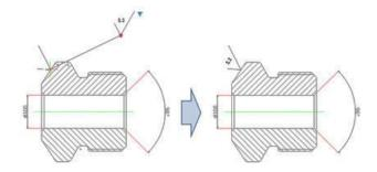
Flip: When you use the "roughness symbol block" to label the spare parts, the symbol is sometimes already in the right position, however, the characters' direction is not right. We need to add the "character flip" function to receive the correct label.
