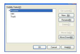
Click the "Invisibility" button in the Visibility tool panel, select truck and car, make them invisible in the "roadster" state, as shown in the following picture, after selecting, press enter to confirm. For the state of "Car" and "Truck", set them in the same way.
