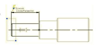
**2.** Add Move Action for keyway: Select the left grip of the linear parameter when moving, stretching the related parameter points. Move the objects of action and select the whole keyway, as in the following picture.
