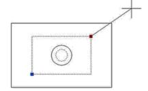
**6. Scale Type:** There is "Scale Type" in the Scale Action Properties. The default value is "XY Scale". If you choose "XY Scale", the dynamic block scales whenever the scale grip moves to X axis or Y axis. If you choose "X Scale", it scales only when the grip of the scale moves to X axis. Same, when you choose "Y Scale".
