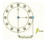
Exit from Block Editor, Drag the grips of the Access hole Block again, you can see, that after the change from Linear Parameter to Polar Parameter, we can drag the grip to scale the dynamic block in any direction.
