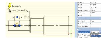
**3.Add the stretch rightwards action for the keyway and realize chain action:** Select the "Distance" linear parameter and modify the chain action of prosperity from "NO" to "Yes" as the following picture shows:
