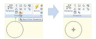
**3.** Insert block: Save and exit block editor, insert the block in the model. You can realize, base point becomes the insert point of the block after adding the base point parameter. Please note, if you set an insert point via the block define dialog box, and add a base point parameter as well, the base point is the default insert point.
