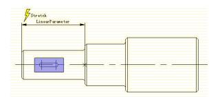
**3. Modify distance multiplier of action:** Select Move Action and modify the default value from 1 to 0.5 in the property of the distance multiplier, save and exit the block editor.
