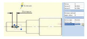
3. Test dynamic block: Exit from block editor, drag stretch grip to stretch the keyway, as shown in the picture.
