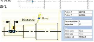
Select the Dynamic Block and then move the right side grip. You will find it can only move in the direction of 30°as it is shown in the follow picture. The direction of action can change according to the Angle Offset.
