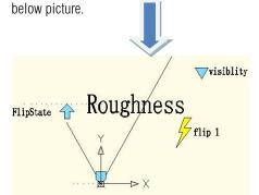
Use the same method to add a pair of flip parameter and action of the vertical direction, as shown:
