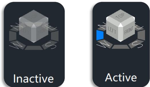
**Cube:** It is in the top right corner of the drawing area over the model, and shows the current viewpoint of the model. When moving the cursor over it, you are able to click the faces, corners or edges to change the views conveniently, as well as click on the cube and drag it to roll the current view.
