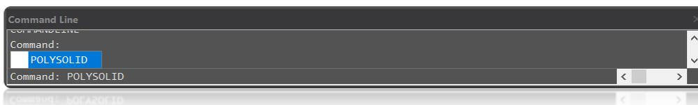
After inputting the PLOYSOLID command, you will get 4 options (Object, Width, Height, Justification) in the command line and dynamic input box.
