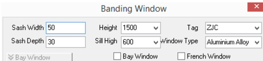
Enter parameter in the above dialog box. If the bay window check box is not checked, the dialog box parameter is used to create ribbon window. The command line prompts:
