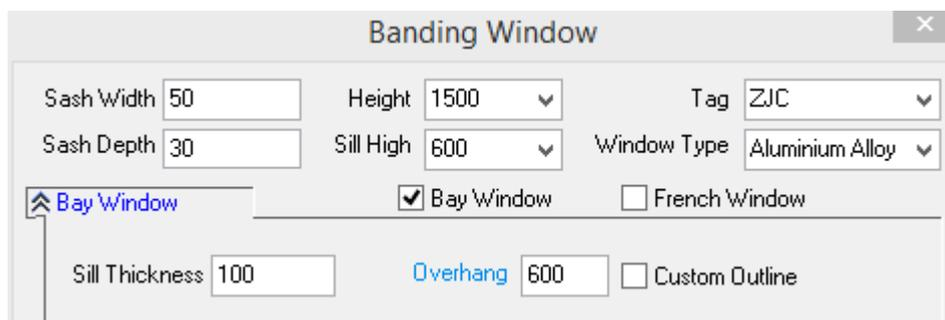
Sideboard is added to the right side of the corner bay window, and the "Overhang" is 600. After the execution of the command, the effect drawing is as shown in the right picture below.
