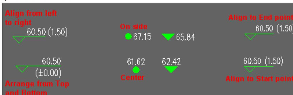
We can double click the elevation object to enter the in-place edit mode, under which we can directly modify the elevation value as follows:
