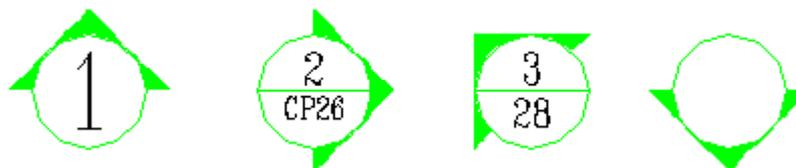
As shown in the above picture, when we check "Viewport Index", we can draw viewport index like this. The feature of it is only one arrow direction is provided. The Viewport Index can index content with any viewport number on other drawings with any sheet number. If the tag or Drawing No is blank, the blank text area will be provided for user to add text in it in the future.
