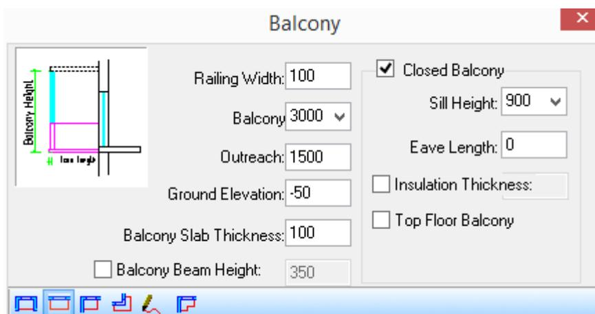
The tool bar at the bottom provides 6 methods to draw the balcony, there are "Concave Balcony", "Rectangle Triangle Balcony", "Internal Corner Balcony", "Offset Drawing along Wall", "Custom Draw", "Select Existed Path to Generate". After the check box "Balcony Beam Height:" is checked, user can enter the value for it to create balcony of beam type.
