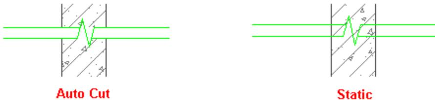
After the above mentioned style is changed, the double break line to be drawn later will be influenced. The existing double break lines will be updated to the current style. When the style is set as double line, the effect of double break line in the above picture will change as follows:
