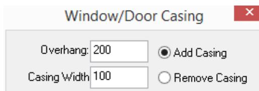
The radio box "Add Casing" in the dialog box is clicked by default. User can click the radio button of "Remove Casing" instead. After setting the parameter "Overhang" and "Casing Width", please move the cursor to the drawing area. Then the interaction in the command line is as follows:
